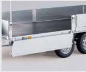
Steel Drop Sides Removable drop sides, tailboard and headboard.
