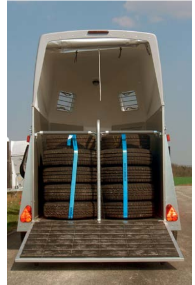
The tyres simulated the horse's weight
